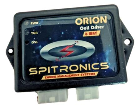
The *Orion Coil Driver* is a quality high performance spark generator designed for basic coils without built-in drivers. The Mercury3 ECU can drive smart coils with built in drivers directly but you have to use the external Orion coil driver for basic coils. Orion2 can do up to 6 Basic coil drivers but in some cases, it is better to use the external coil driver with the positive drivers. This may free up more negative drivers for other tasks.
